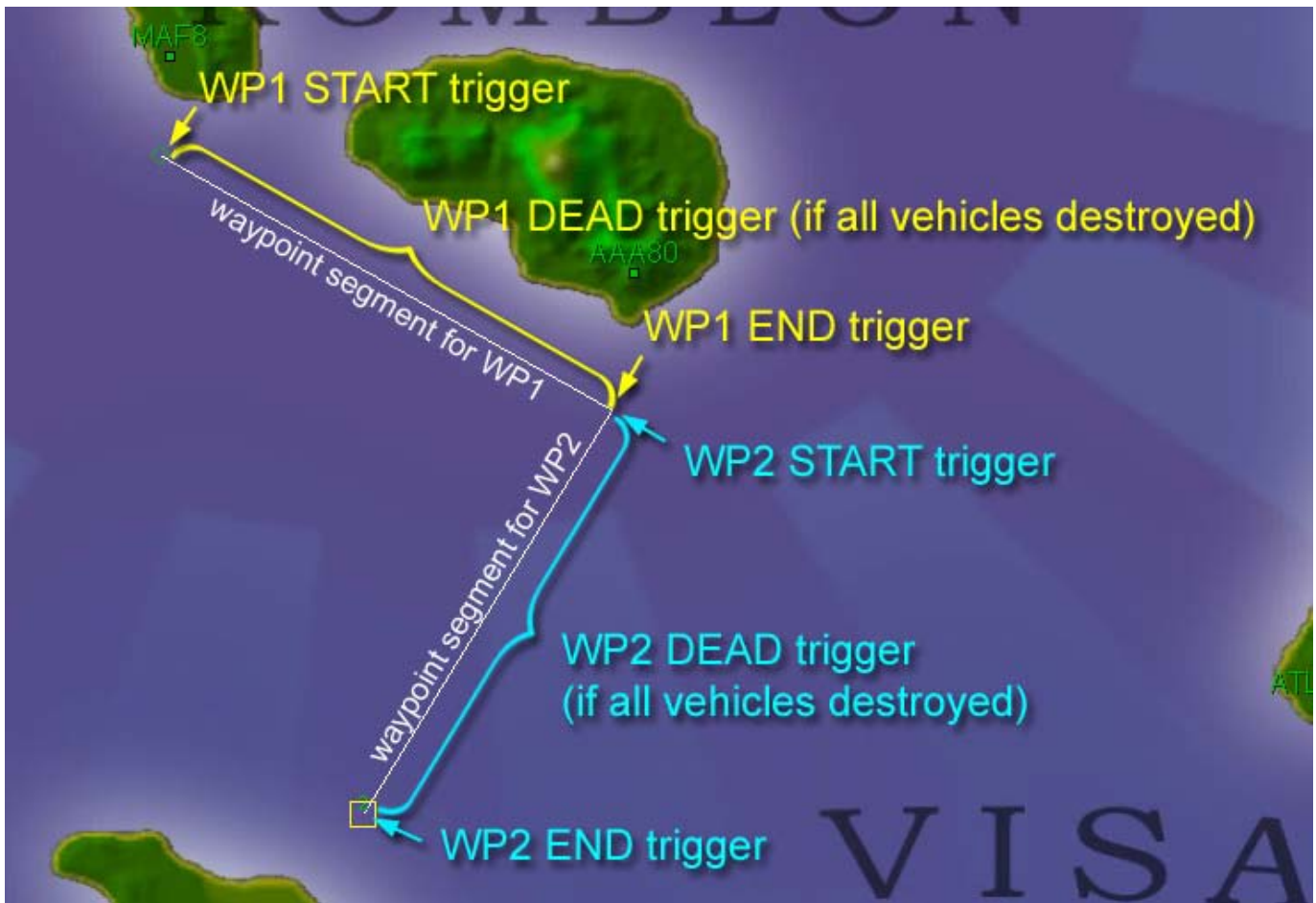
Figure 8 – Locations of Waypoint Triggers: Each waypoint segment has three trigger types. The START and END triggers are always activated at the start and end of the waypoint segment, respectively. The DEAD trigger for a waypoint segment is only activated if the last remaining vehicle is destroyed within the waypoint segment.
